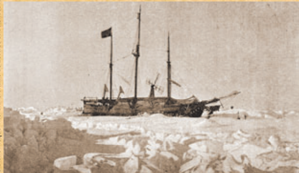
The boat Fram , built by order of Fridtjof Nansen. Designed to withstand the pressure of the ice, Nansen used it during his second expedition to the Arctic.
